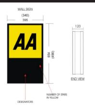
These stylish signs are manufactured in aluminium, with acrylic panels. All signs can be internally illuminated and come with 4,000mm of cable for connection.
