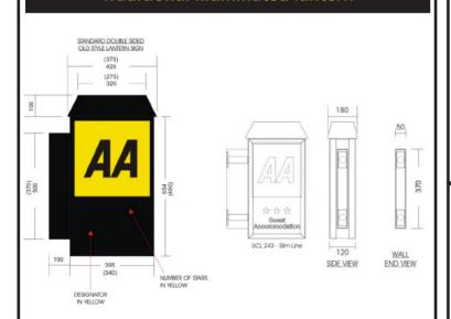
Manufactured in aluminium, the traditional illuminated lantern comes complete with fixing brackets. They can be internally illuminated and come with 4,000mm of cable for connection. With the option available to display the traditional AA logo, these signs are useful on buildings where planning permission for modern designs has been refused.
