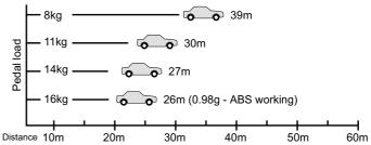
Fade test: pedal load required for a moderate (34m/.75g) stop: 11kg at start of test, 14kg at end of test (*Ideal brakes show no change*)
