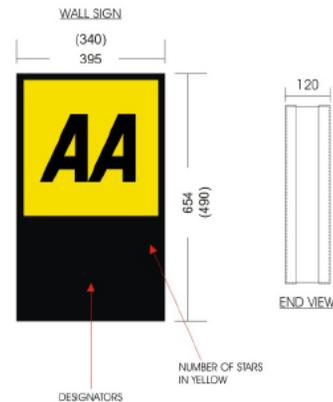
These stylish signs are manufactured in aluminium, with acrylic panels. All signs can be internally illuminated and come with 4,000mm of cable for connection.
