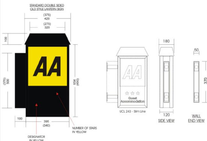
Manufactured in aluminium, the traditional illuminated lantern comes complete with fixing brackets. They can be internally illuminated and come with 4,000mm of cable for connection. With the option available to display the traditional AA logo, these signs are useful on buildings where planning permission for modern designs has been refused.
