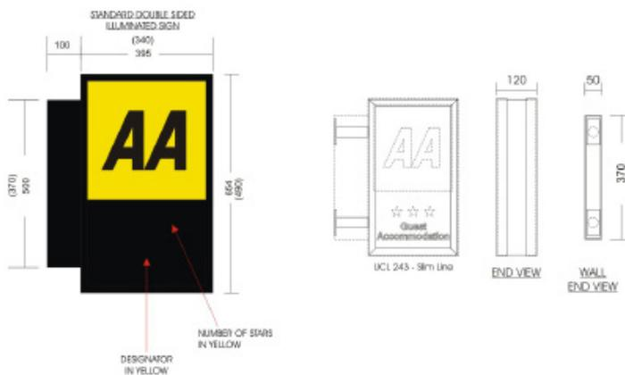
Manufactured in aluminium, these popular signs contain acrylic panels showing the widely recognised AA logo, the establishment designator and star rating. Supplied with 4,000mm of cable.
