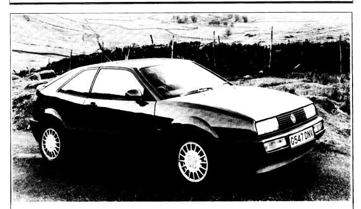
VOLKSWAGEN'S new, mean-looking sports coupé is clearly designed to replace the Scirocco, although the importer insists that there is no plan imminent to withdraw the older model. The Corrado 16V's mechanicals are an amalgam of components from existing products — the power unit is from the higher-powered Golf GTI and the 'passive-steer' rear suspension is similar to the new Passat's.
