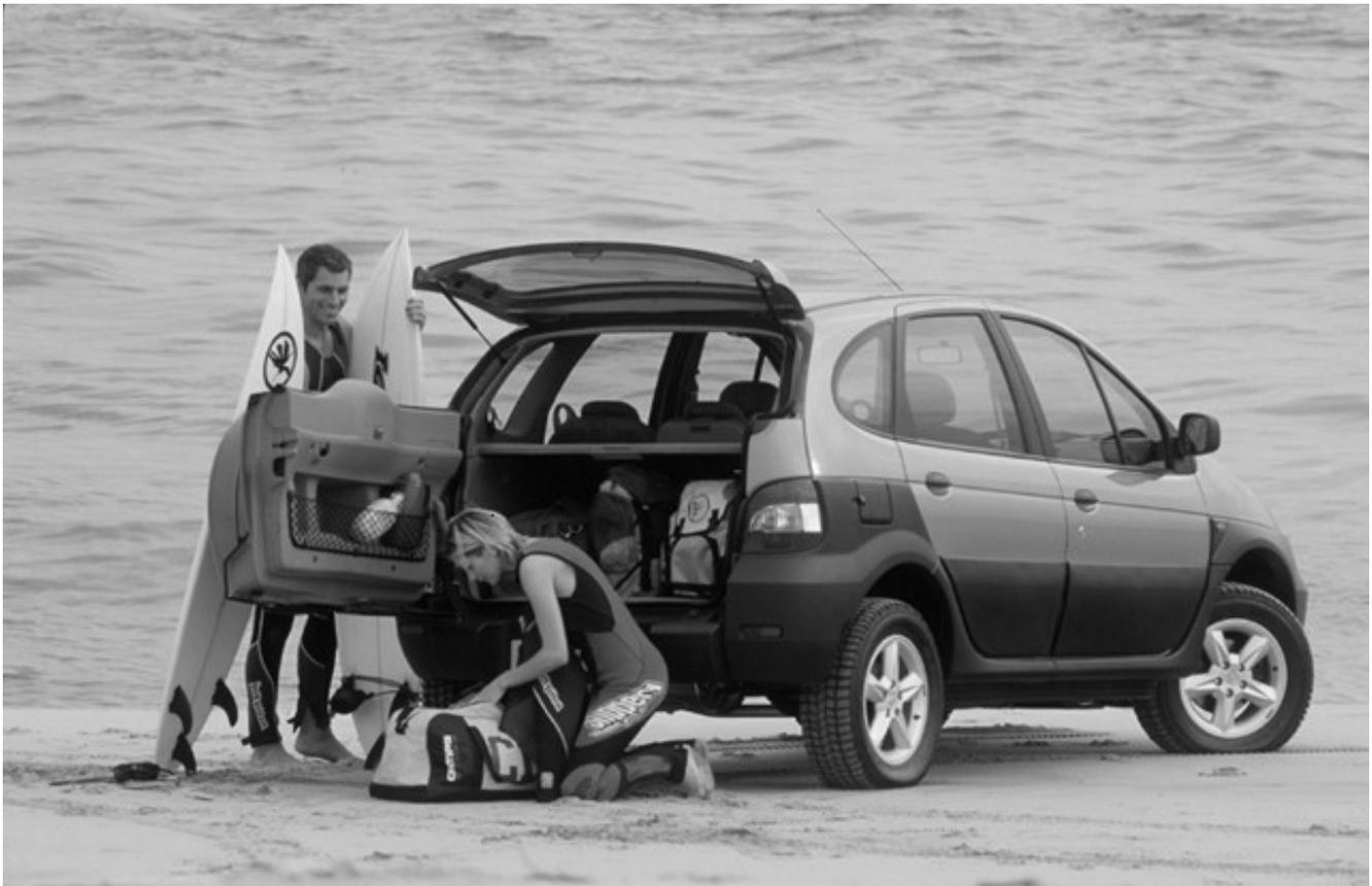
split-level affair, with its electric release also operating a separate lift-up glass hatch.
