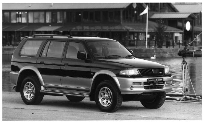
ITSUBISHI SAYS THAT ITS NEW Challenger is whatever you want it to be, but the company is promoting it as a sports utility vehicle, because it slips rather neatly into the UK line-up between two of the models on which it's based. It has the engines, ladder-frame chassis and front suspension of the beefy Shogun, and the rear springing of the "lifestyle" L200 Double Cab.
