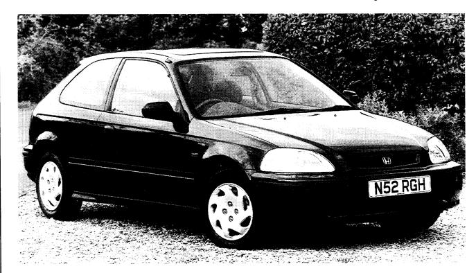
HESE CIVICS DIFFER FROM THE Swindon-built five-door by being made in Japan and having different engines, too. There's also a stylish coupé and a CRX, but here we look at the 1.5 manual and the 1.6 automatic – both with 115bhp on offer. Where they differ is that the Auto uses Honda's new Continuously Variable Transmission (CVT) even though a conventional torque converter "stepped" auto, box is also available.
