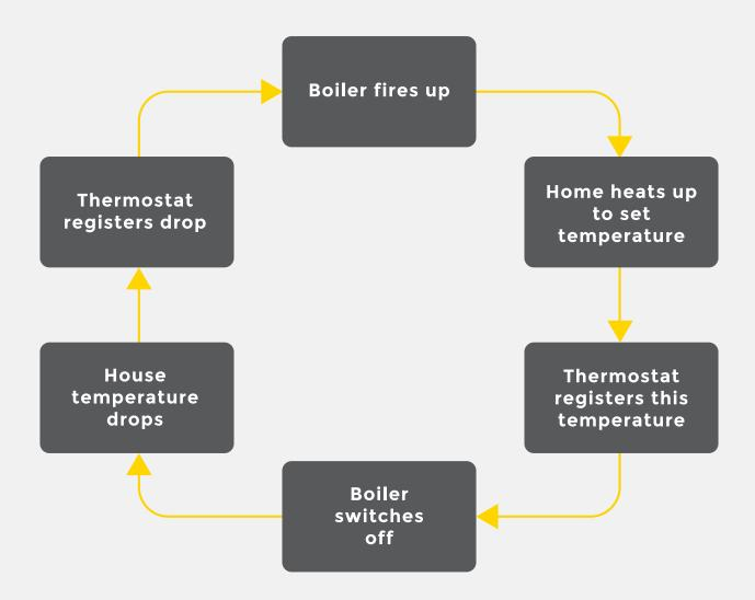
The thermostat works with the boiler, using the following process to keep the home warm when the programmer turns the boiler on.
