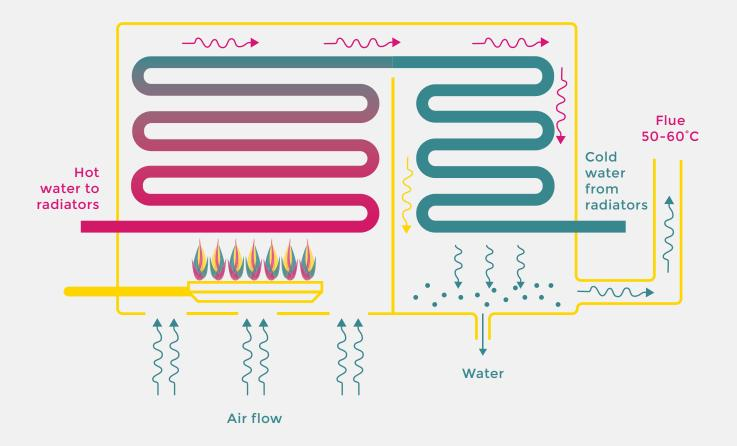
The main function works the same way as the non-condensing boiler, but the waste gases are routed through a second heat exchanger, cooling it back into a liquid state known as condensate.
