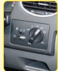
**Q13. Show me how you switch your headlight from dipped to main beam and explain how you would know the main beam is on whilst inside the car.**
